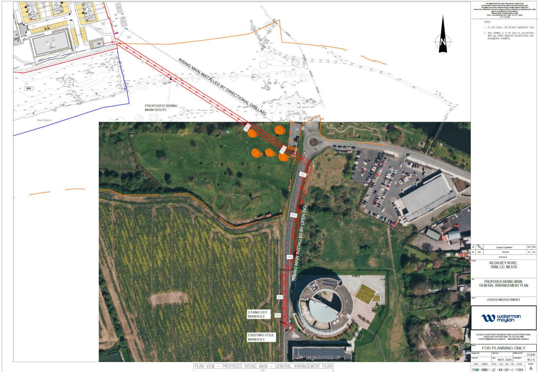
Figure 19. Proposed rising main general arrangement plan
